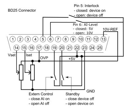
All digital outputs are OC outputs with a pull-up resistance after + 5 V. All analog inputs and outputs can be operated in 0-5 V or in 0-10 V mode.
